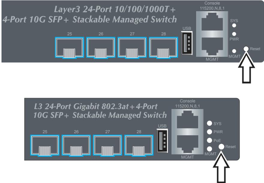
Figure 12-1: SGS-6341-24T4X and SGS-6341-24P4X Reset Button
